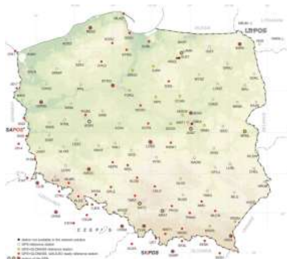
Fig. 10. Distribution of ASG-EUPOS permanent GNSS reference stations ( http://www.asgeupos.pl/webpg/graph/dwnld/map_en_dwnld.jpg 2014)
