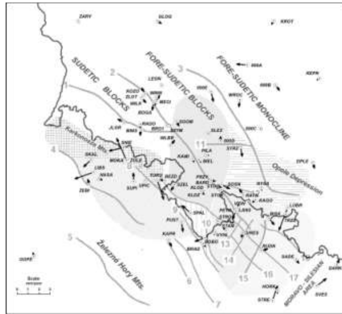
Fig. 14. Vectors of horizontal intraplate velocities (ITRF2008 reduced with ITRF2008 plate-motion model) (Kaplon et al., 2014)
