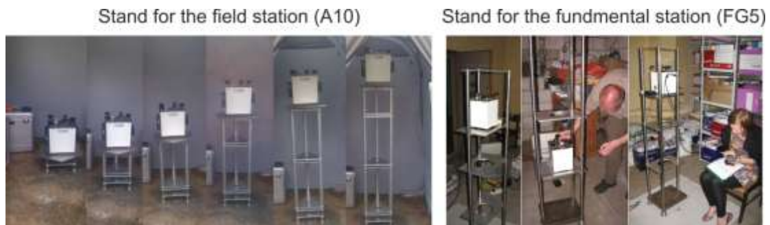
Fig. 20. The stand constructed by WUT (left) and IGiK (right) for vertical gravity gradient determination at field station and laboratory station, respectively
