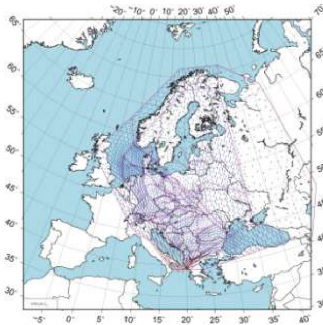
Fig. 10. Strain directions ( S_{MAX} ) obtained using Finite Element Method modelling
