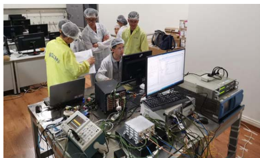
Fig. 12 Satellite to ground S-band interface compatibility test
