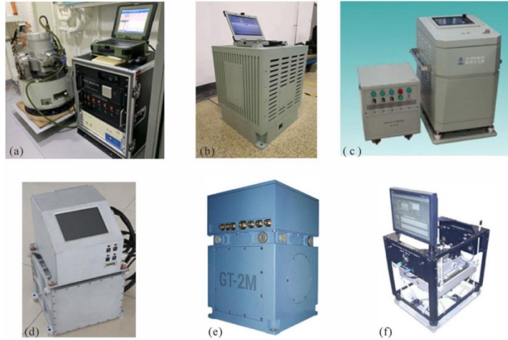
Figure 14. Marine relative gravimeters: a CHZ-II; b ZL11; c SAG-2M; d SGA-WZ; e GT-2M; f LCR (Yuan et al., 2018)
