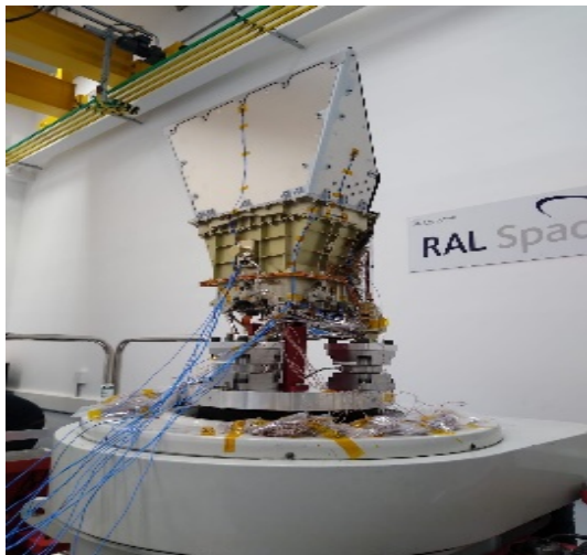
Fig. 5 SXI STM on a shaker table at RAL, UK
