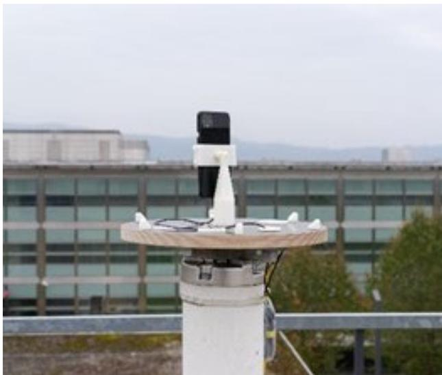
Figure 4.22: Experimental setup for the test of the Google Pixel 4XL for tropospheric studies. For the tests, the smartphone was covered by a radome.
