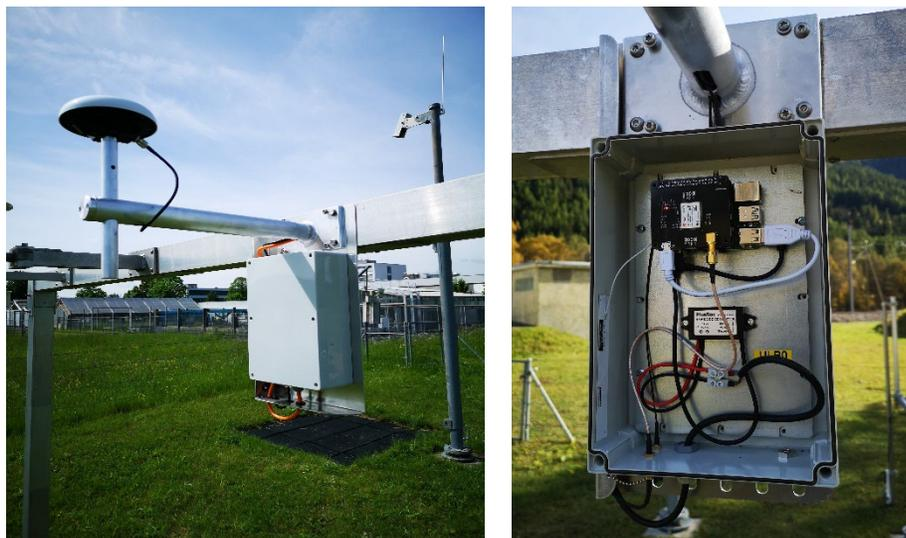
*Figure 4.31: Left: Full MPG-NET prototype setup installed at the SMN-site Zurich-Affoltern (REH). Right: Interior of the box containing the main parts of the MPG-NET data logging system.*
