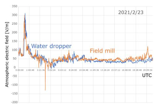
Comparison between water-dropper device and field mill device on 23 February 2021. Two records are well coincided
