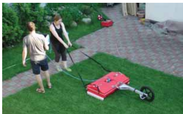
Deployment of GPR with various antennas
