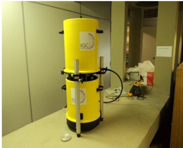
Fig. 2.5 Absolute gravity meter A10-32
