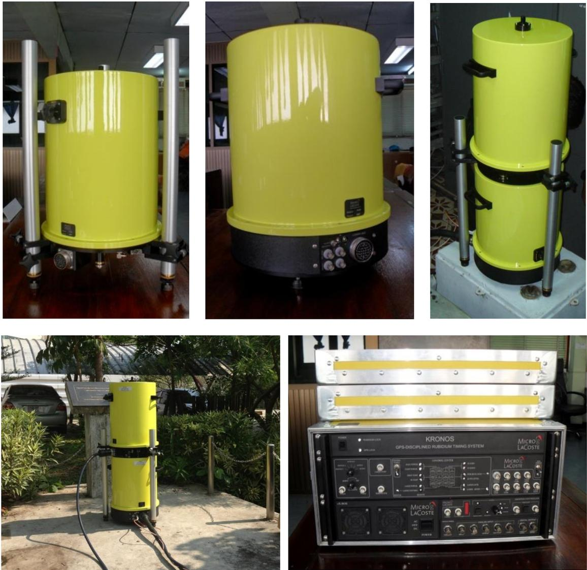
Figure 10 : Absolute Gravimeter “Micro – g Lacoste Model A-10”
