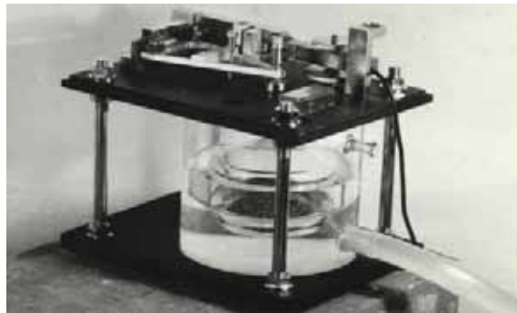
Figure 2. Water-tube tiltmeter (single terminal)
