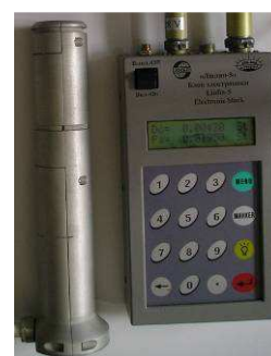
Fig. 5. External view of the dosimetric telescope Liulin-5.
