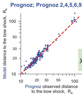
Fitted parameters - magnetopause stand off distance  $r_0$ , nose curvature radius  $R_0$  and bluntness  $b = -8\pi/3 (\pi R_0/D)^2$  - from MP model were used as entry parameters for the bow shock model
