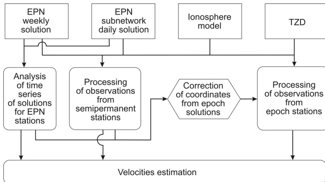
Fig. 1.5.2b. Diagram of GPS data processing strategy for combined processing of permanent and epoch observations
