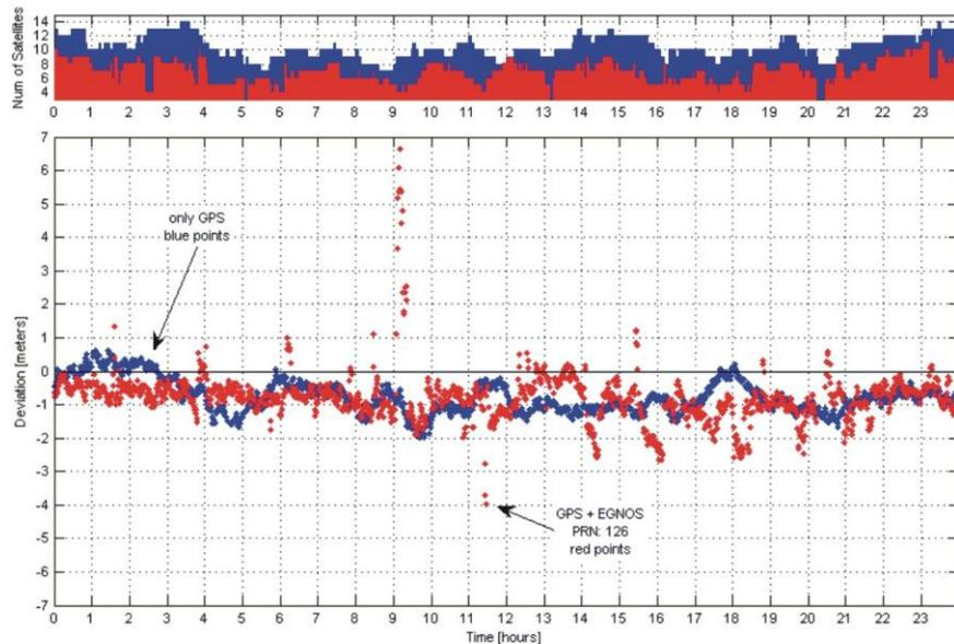
Fig. 4.10.4. The resulted values of Y coordinate for static measurement from 22 May 2007. The upper graph shows the number of observed satellites and the bottom one – the position of the receiver. The blue dots present GPS only measurements and red ones the GPS+EGNOS
