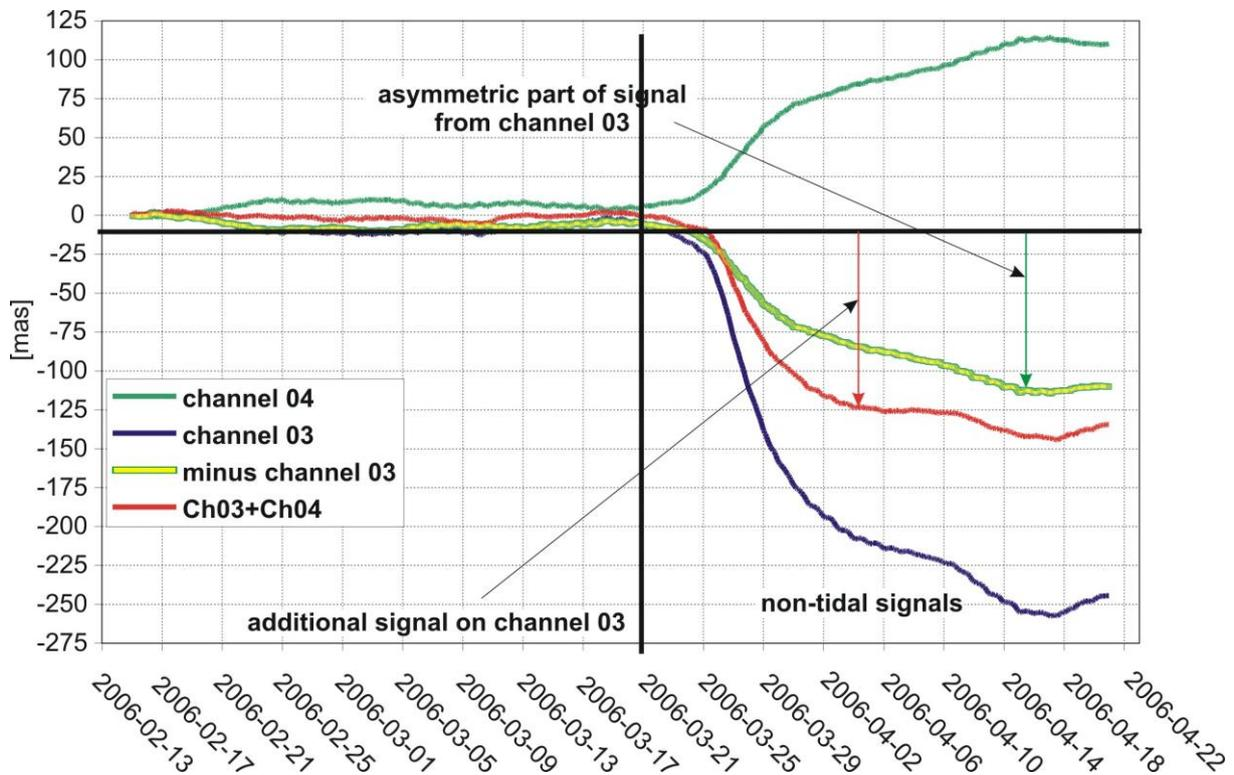
Fig. 2.5.2. Non-tidal signals observed by tube 03-04 in March 2006 in azimuth 148.6 (event 4<sup>th</sup>) after the elimination of tidal and evaporation signals
