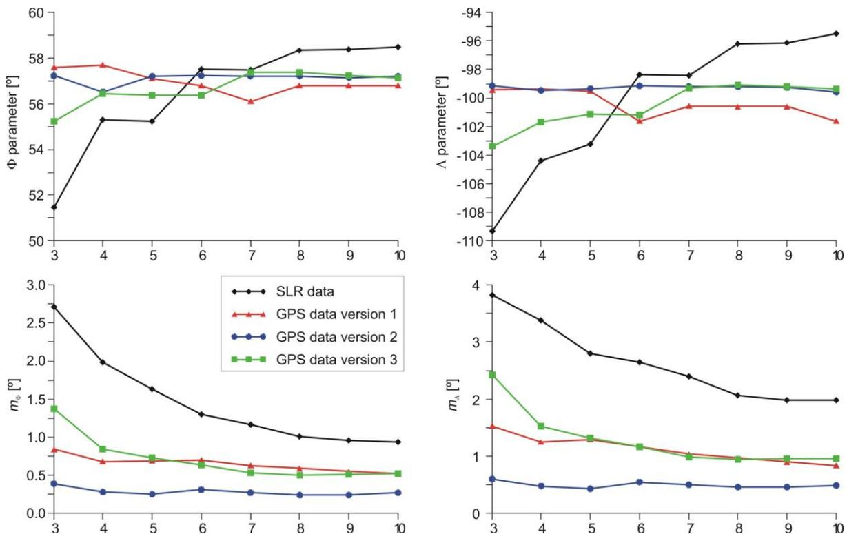
Fig. 3.6.4. Parameters  $\Phi$  (upper left) and  $\Lambda$  (upper right) of the tectonic plate motion and their errors  $m_\Phi$  (lower left) and  $m_\Lambda$  (lower right) estimated from the SLR and GPS techniques (Eurasian plate)
