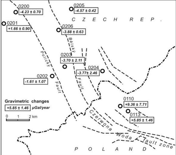
Fig. 3.2.3f. Velocities of gravity changes and their mean errors on network points in 1993–2009
