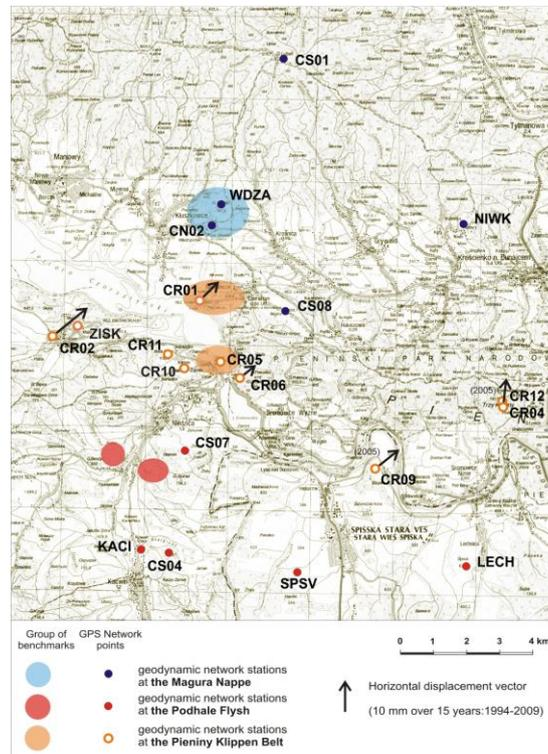
Fig. 3.2.4c. Velocity vectors at selected points at the Pieniny Klippen Belt
