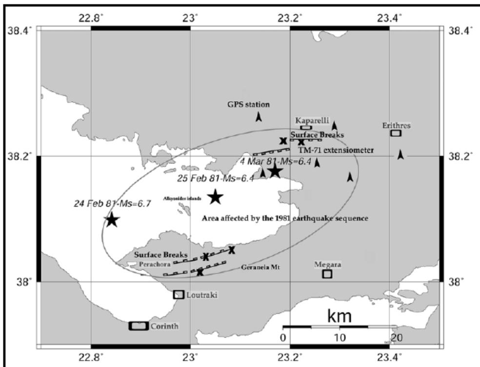
Fig. 3.2.5. Map of Kaparelli test area with epicentres of the 1981 earthquake sequence (stars). X marks show the locations of the TM-71 instrument and black arrows indicate the locations of non-permanent GPS stations installed during 2003. Lines with barbs indicate normal faults that ruptured during the 1981 earthquake sequence
