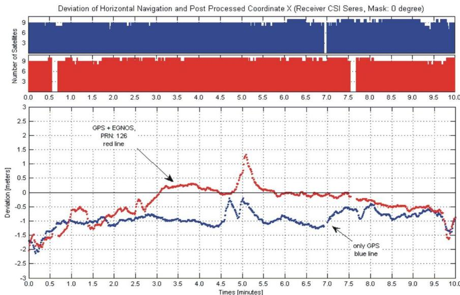
Fig. 4.10.5. The resulted values of X coordinate for static measurement from 17 April 2007. The upper graph shows the number of observed satellites and the bottom one – the position of the receiver. The blue dots present GPS only measurements and red ones the GPS+EGNOS
