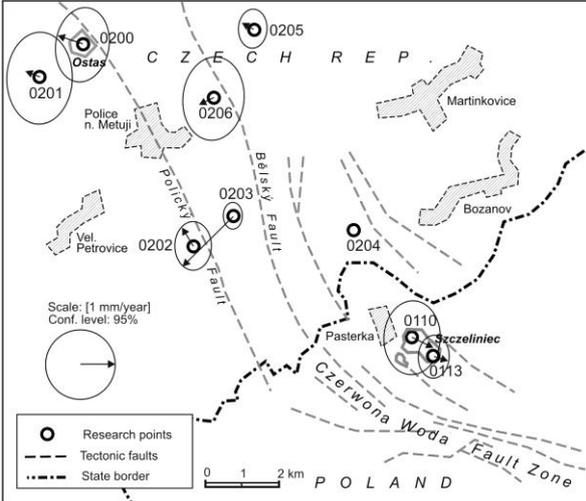
Fig. 3.2.3e. Horizontal velocity vectors and their confidence ellipses at the 95% level
