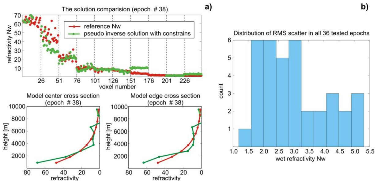
Fig. 4.6.10. a) The intersection through the model, real observed SWDs were used (tomographic solution - grey line, COAMPS reference data – black line); b) The histogram of the RMS of the real data solution with respect to COAMPS reference data (Rohm and Bosy, 2010)
