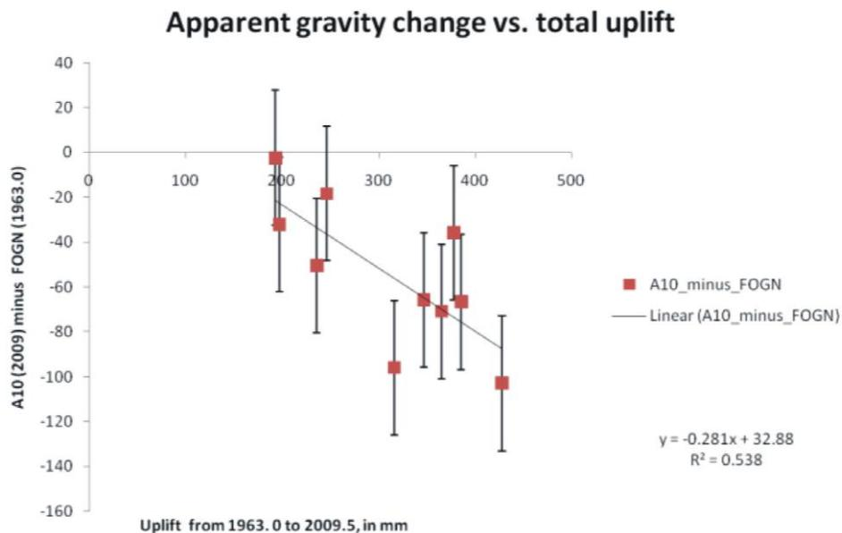
Fig. 3.6.2b. Apparent gravity change at 10 stations of the Finnish Gravity Control Network re-surveyed with the A10-020 in 2009 and 2010 vs. total uplift
