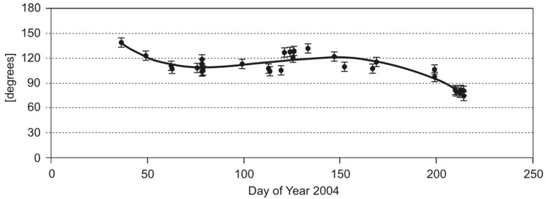
Fig. 4.5.1c. Spin axis of LAGEOS-1 – co-latitude component and the trend function
