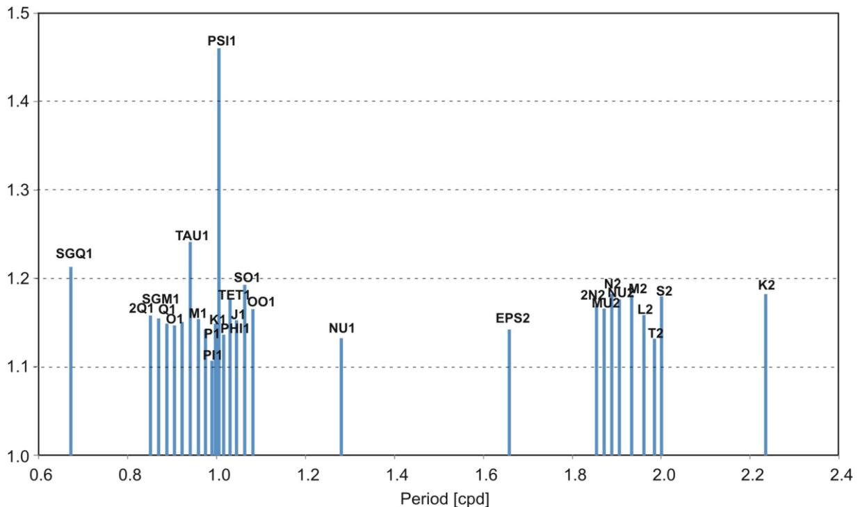
Fig. 3.5.1. Amplitude factors of the empirical tidal model based on observations of the Jozefoslaw Observatory
