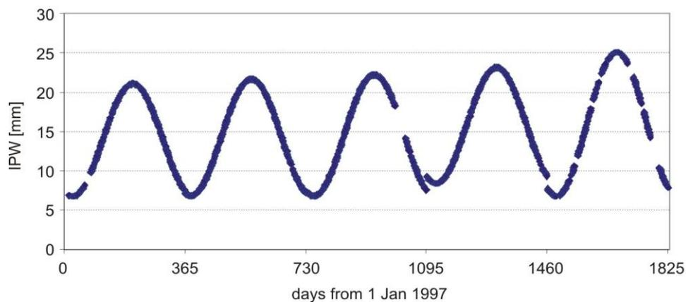
Fig. 4.6.7. Simple model of daily IPW values series (sinusoid + constant) derived from IGS CODE ZTD solution for JOZE 1997–2001
