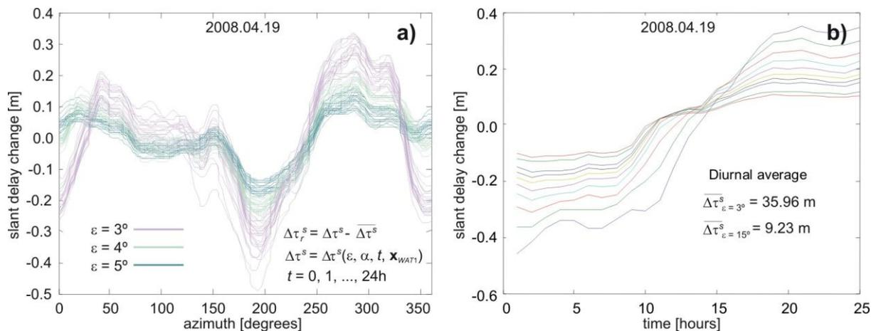
Fig. 4.6.1. Slant delay differences and their azimuth average values for each hour COAMPS forecast a); azimuthally averaged differences of hourly and diurnal slant delays b)
