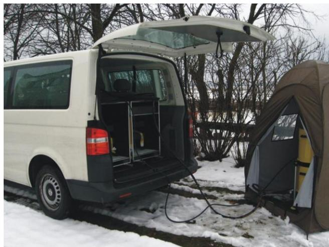
Fig. 2.5.1c. Field survey with the A10-020 using mobile gravimetric laboratory
