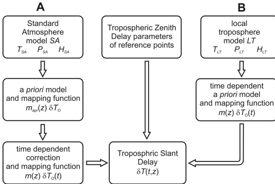
Fig. 4.9.1. The tropospheric delay estimation procedures based on the standard (A) and local (B) atmosphere models for local GNSS networks data processing models
