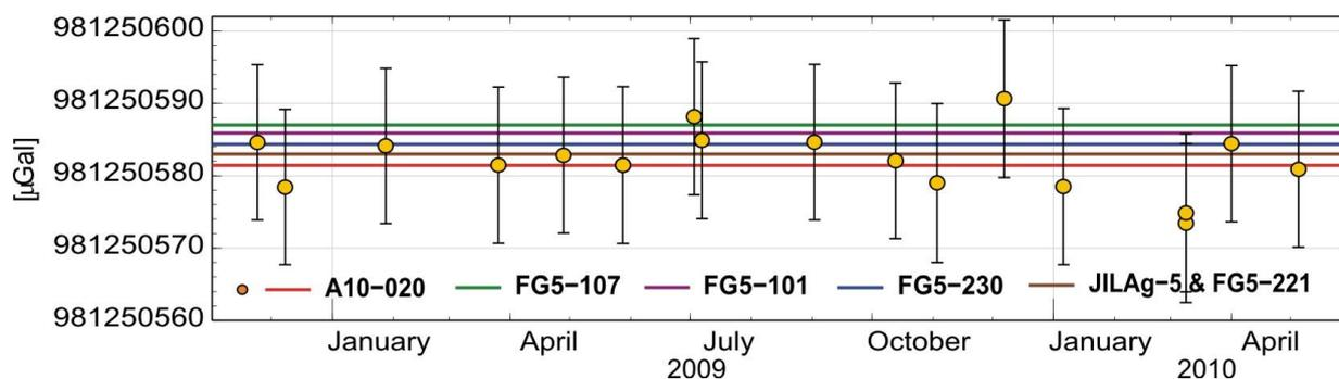
Fig. 2.5.1a. Results of absolute gravity measurements with the A10-020 at Borowa Gora laboratory station
