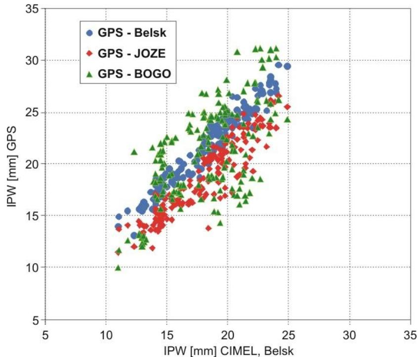
Fig. 4.6.5. IPW from sunphotometer in Belsk and GPS data ‘in situ’, JOZE (33 km distance) and BOGO (73 km) in September 2009
