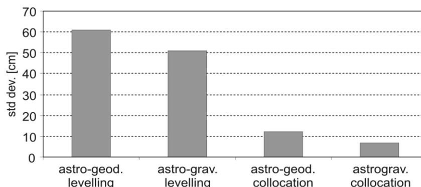
Fig. 2.2.4. External accuracy of astro-geodetic and astro-gravimetric geoid models developed, represented by the standard deviation of their fit to the GPS/levelling geoid at the sites of the POLREF network
