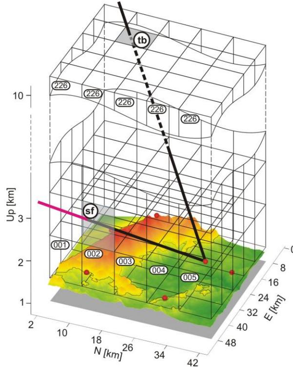
Fig. 4.6.9. The ray path in consecutive voxels. Two cases are considered, the first when the ray is coming out of the model's side face (sf), and the second, when ray is coming out of the model top boundary (tb). Model presented here has 25 voxels in 10 layers (Rohm and Bosy, 2009, 2010)
