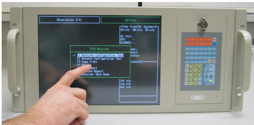
Fig. 4.4.2. New TTS-4 receiver with touch-control screen
