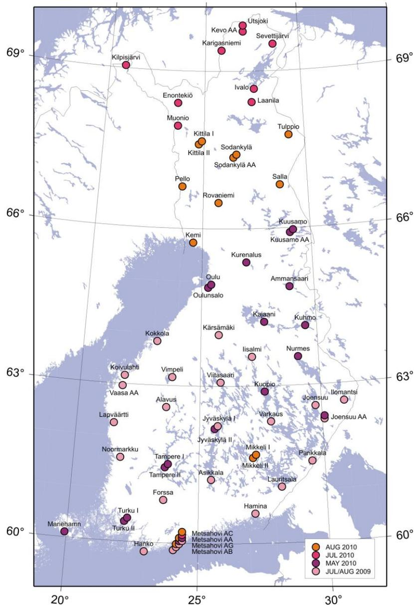
Fig. 2.3.2. Stations of the Finnish Gravity Control Network re-surveyed with the A10-020 in 2009 and 2010; the laboratory-type absolute-gravity sites where comparisons with measurements with the FG5-221 were made have two letters after the name
