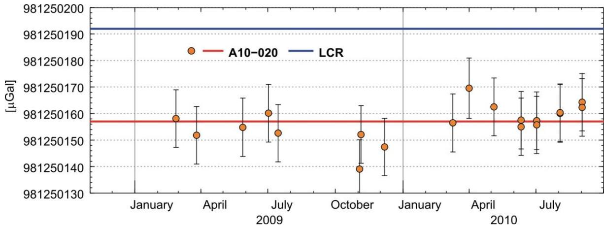
Fig. 2.5.1b. Results of absolute gravity measurements with the A10-020 at Borowa Gora field station
