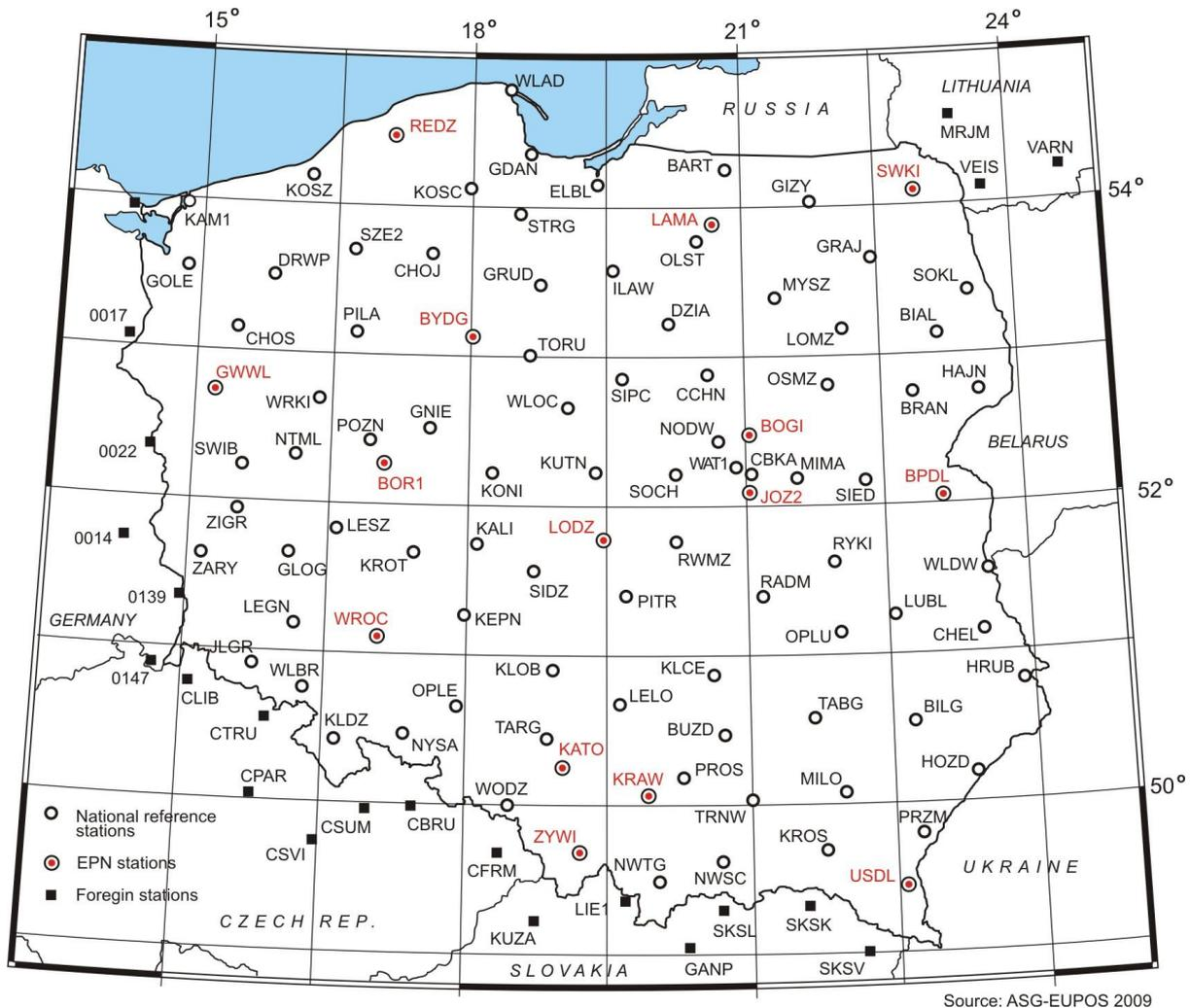
Fig. 1.5.1. Reference stations included in ASG-EUPOS ([www.asgeupos.pl](http://www.asgeupos.pl))
