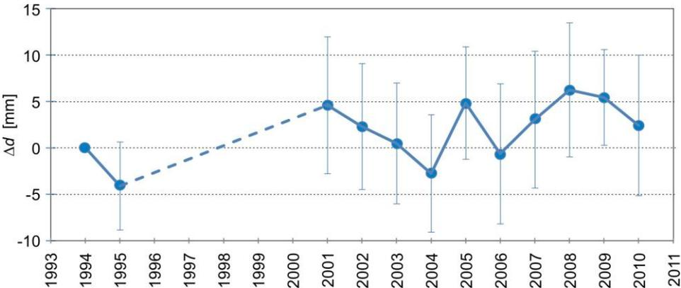
Fig. 3.2.4a. Distance changes between Podhale Flysch and Magura Nappe
