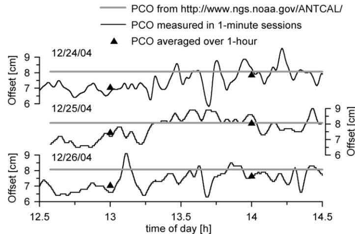
Fig. 4.5.6. Comparison of the results of the mean phase centre offset obtained from the observations with the results of NGS calibration
