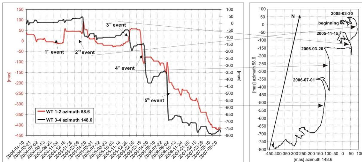
Fig. 3.5.2. Non-tidal signal observed by long water-tube tiltmeter in period 2004–2007
