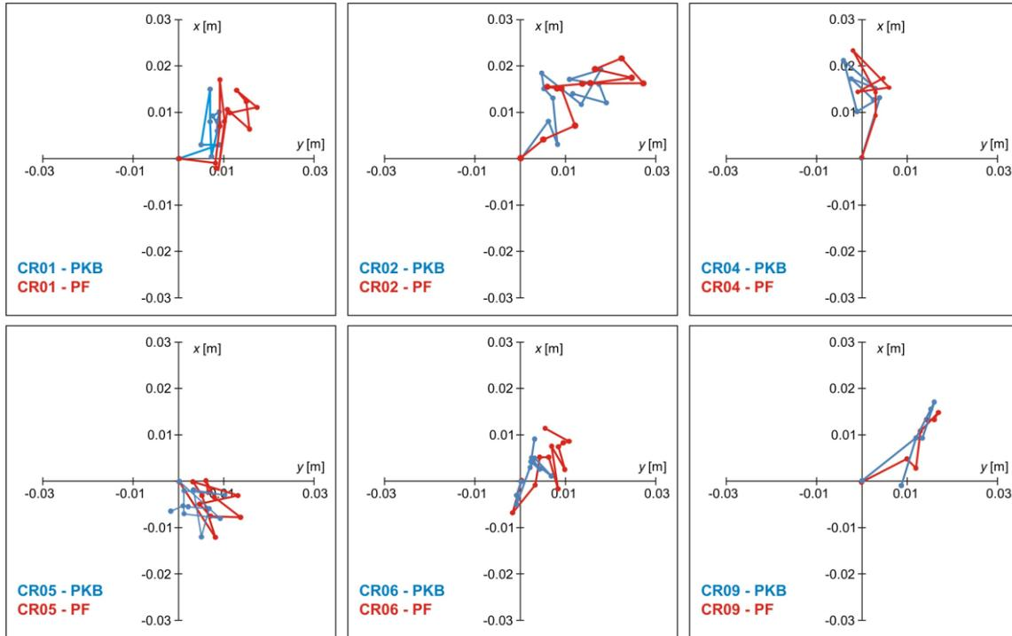
Fig. 3.2.4b. Points movements within the Pieniny Klippen Belt PKB (relative the Magura Nappe – blue, and Podhale Flysch PF – red)
