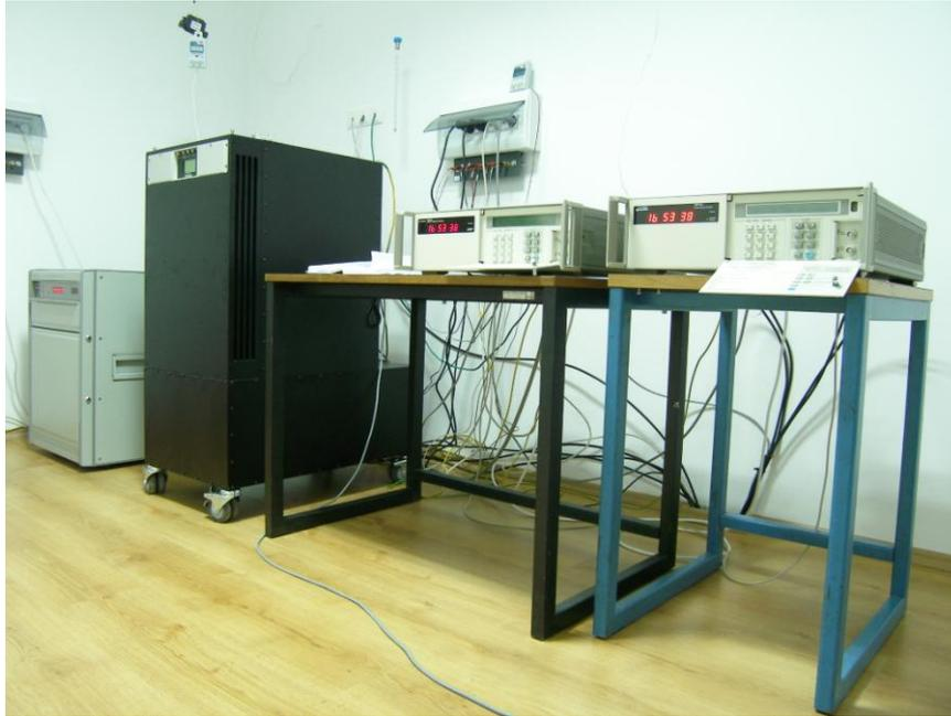
Fig. 4.4.1. Clock ensemble at AOS; from the left: Russian CH1-75A, and then American Symmetricom SigmaTau
