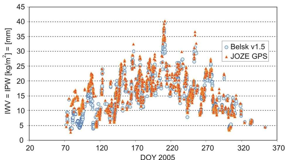
Fig. 4.6.4. Integrated Precipitable Water values validated by independent technique: sunphotometer CIMEL CF-318 (Central Geophysical Observatory, Belsk near Warsaw, 33 km from JOZE) – results shown for 2005
