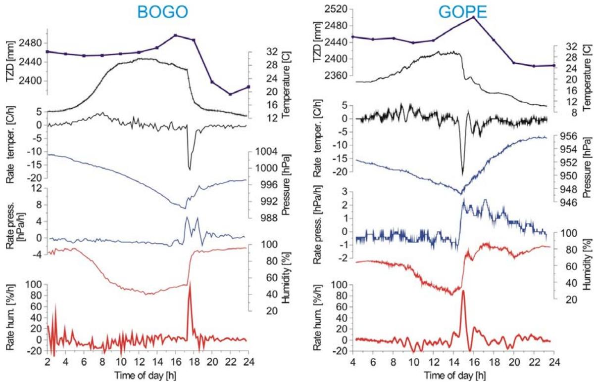
Fig. 4.6.1. Dynamics of variations of meteorological parameters and TZD when the atmospheric front was passing over BOGO and GOPE stations in 27 August 2001
