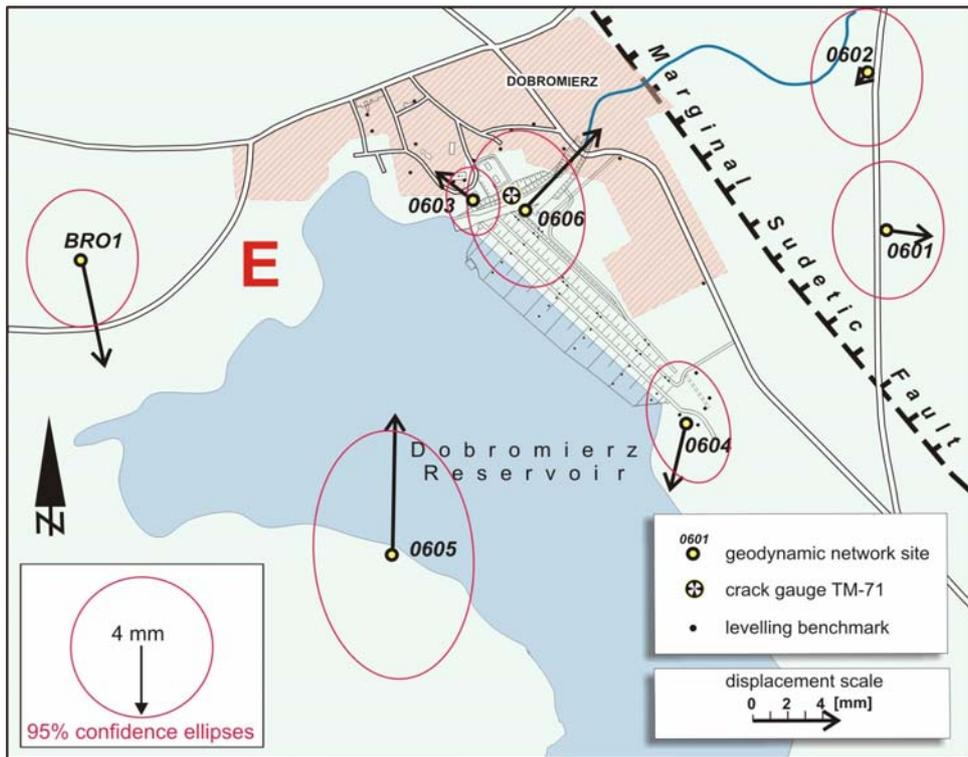
Fig. 3.2.7. Results of geodynamic research in 2001-2005 in Dobromierz Dam polygon
