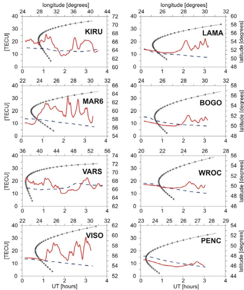
Fig. 4.7.4. Temporal TEC variations along individual satellite passes for PRN14 observed at different stations on quiet (blue) and disturbed (red) day (Krankowski et al., 2004b)
