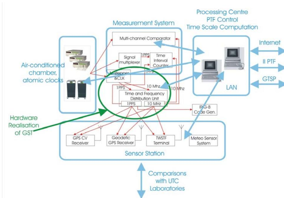
Fig. 4.4.6. Simplified diagram of Galileo Precise Time Facility
