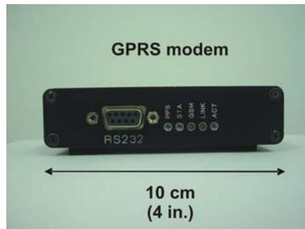
Fig. 1.5.6. GPRS modem designed by Biatel
