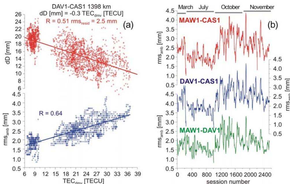
Fig. 4.7.12. Variations of vector length and uncertainty of ambiguity estimation versus TEC (a), and time series of uncertainties of ambiguity estimation for the periods of different stability of ionosphere (b)
