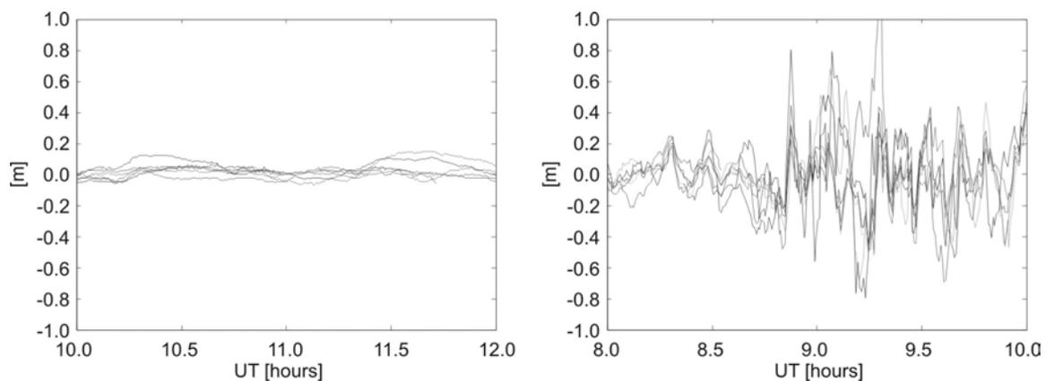
Fig. 4.7.9. DD ionospheric correction residuals with respect to the reference “truth” during the analysed quiet and stormy periods (COLB-LEBA, 121 km) (Wielgosz et al., 2005b)
