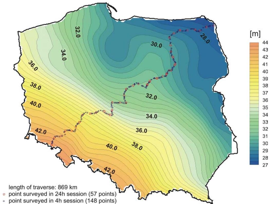
Fig. 2.2.3. GPS/levelling control traverse
