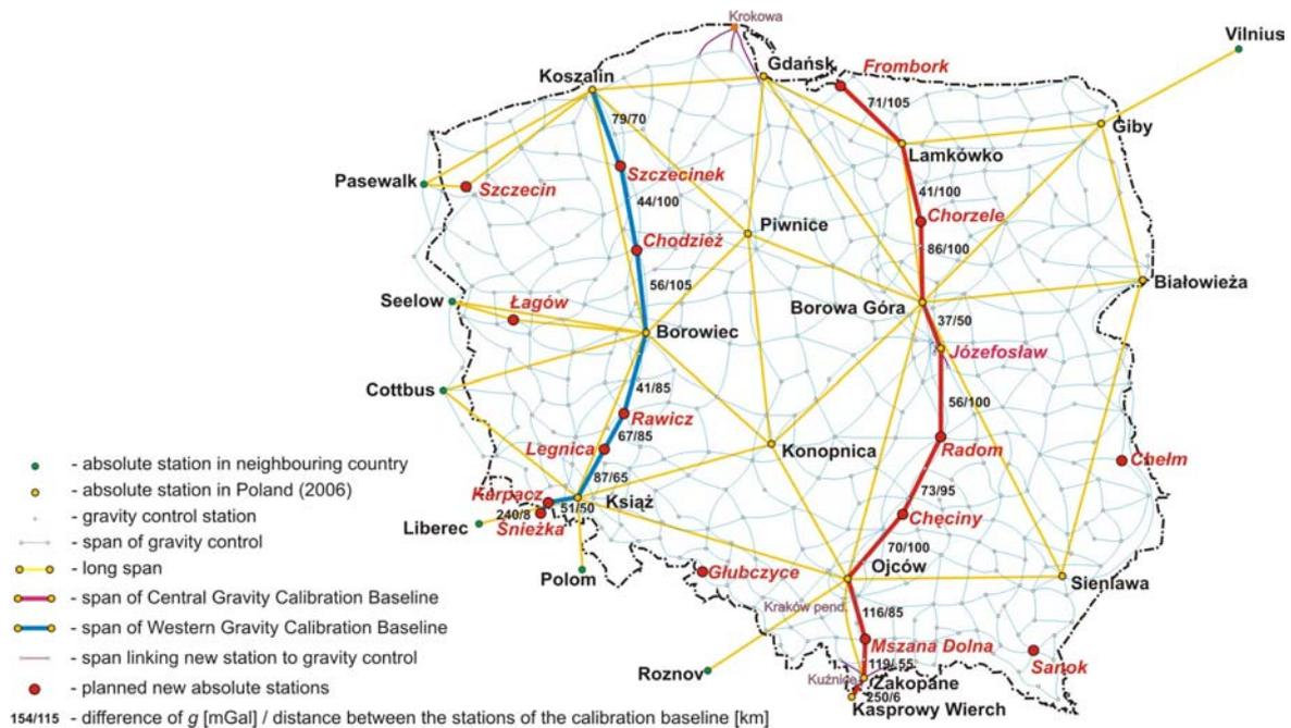
Fig. 2.4.2. Modernised Gravity Calibration Baseline in Poland (2006 – project)
