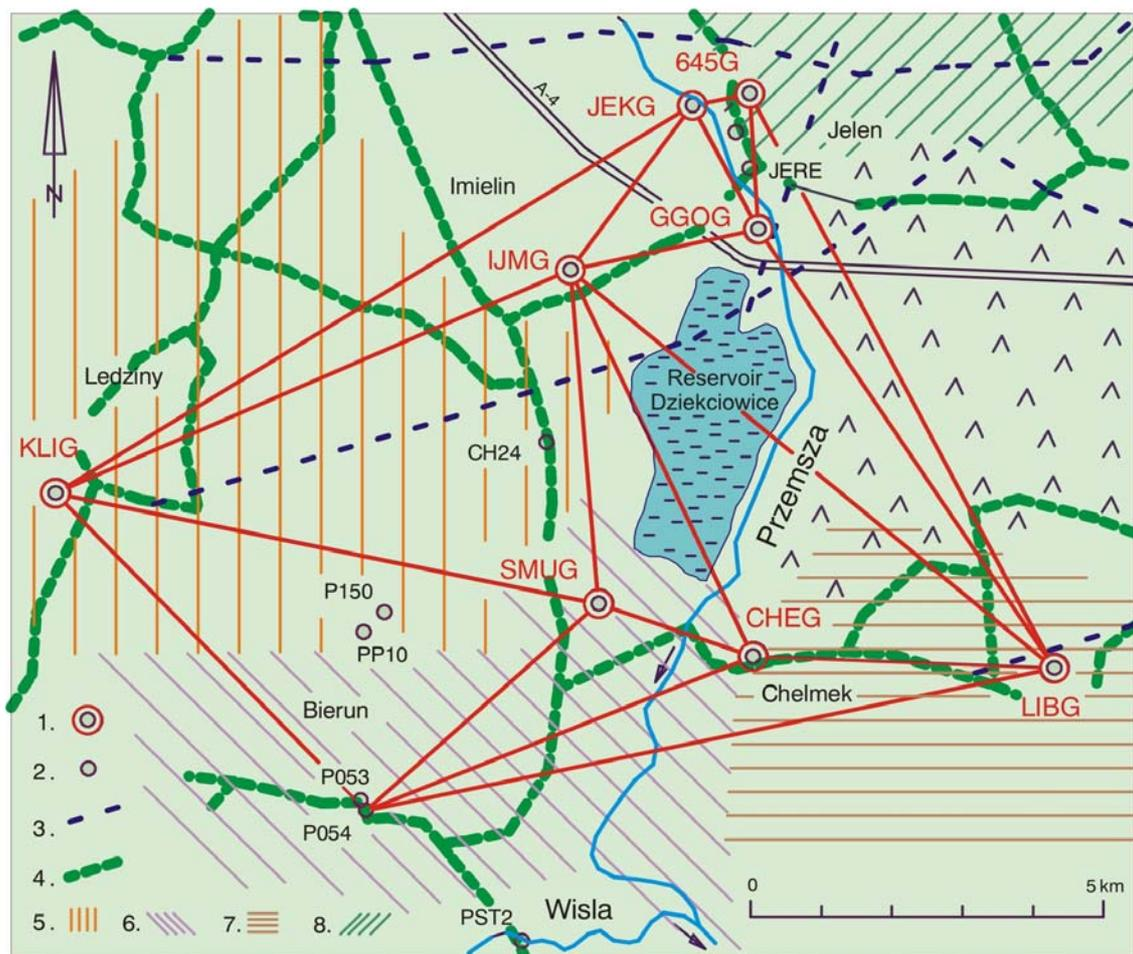
Fig. 3.2.11. The research geodynamic network along the “Przemsza” river.
