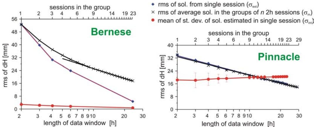
Fig. 4.5.7. Standard deviations of the GPS-derived vertical component provided by processing softwares, and estimated by statistical analysis of time series of GPS solutions
