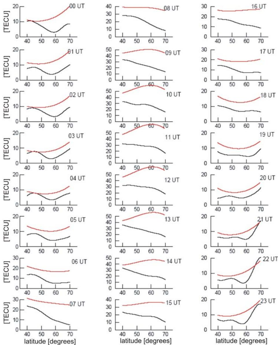
Fig. 4.7.2. Comparison of latitudinal profiles of GPS-derived TEC (black) with IRI model (red) for 15 December 1999 (Wielgosz et al., 2004a)
