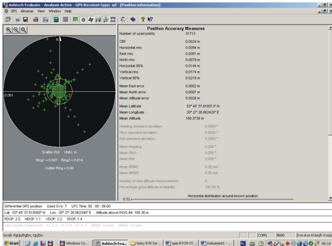
Fig. 1.5.7. The results of the RTK test lasting for nine hours with very optimistic continuity of data transmission and very good positioning accuracy
