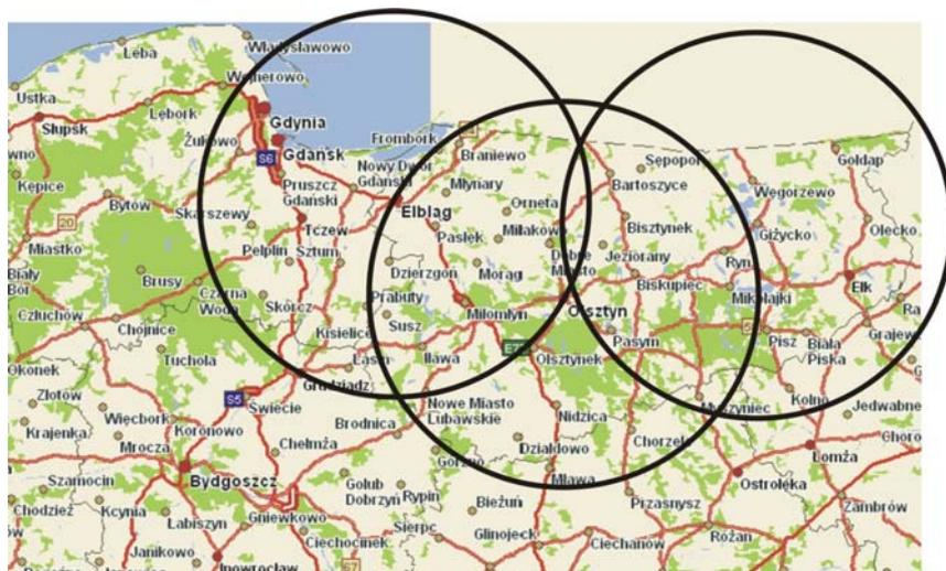
Fig. 1.5.5. Network of 3 reference stations and theoretical range of the DGPS/RTK services in North-East Poland
