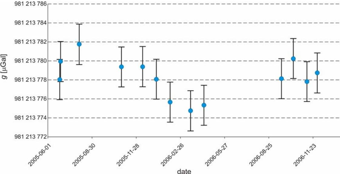
Fig. 2.3.2. Absolute gravity measurements at Jozefoslaw with FG5 No 230
