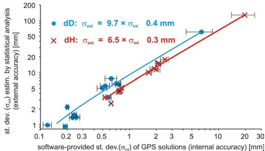
Fig. 4.5.8. Correlation between the external accuracy  $\sigma_{\text{ext}}$  and the internal accuracy  $\sigma_{\text{int}}$  of GPS solution for distance (D) and vertical component (H) provided by the *Bernese* software
