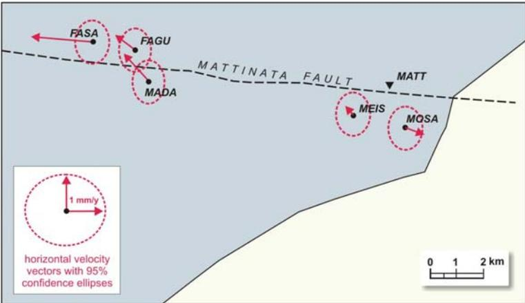
Fig. 3.2.14. Horizontal velocity vectors of Gargano network sites
