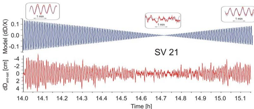
Fig. 4.5.11. Time series of modelled and observed variations of satellite-antenna distance for PCV determination
