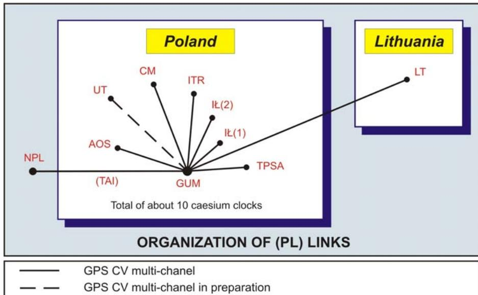
Fig. 4.4.1. Configuration of laboratories contributing to TA(PL)
