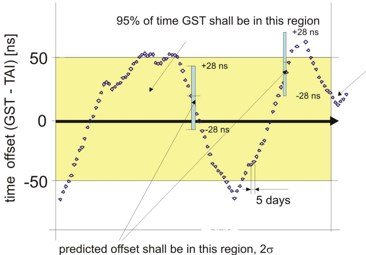
Fig. 4.4.5. Realization of the Galileo System Time by Galileo Time Service Provider
