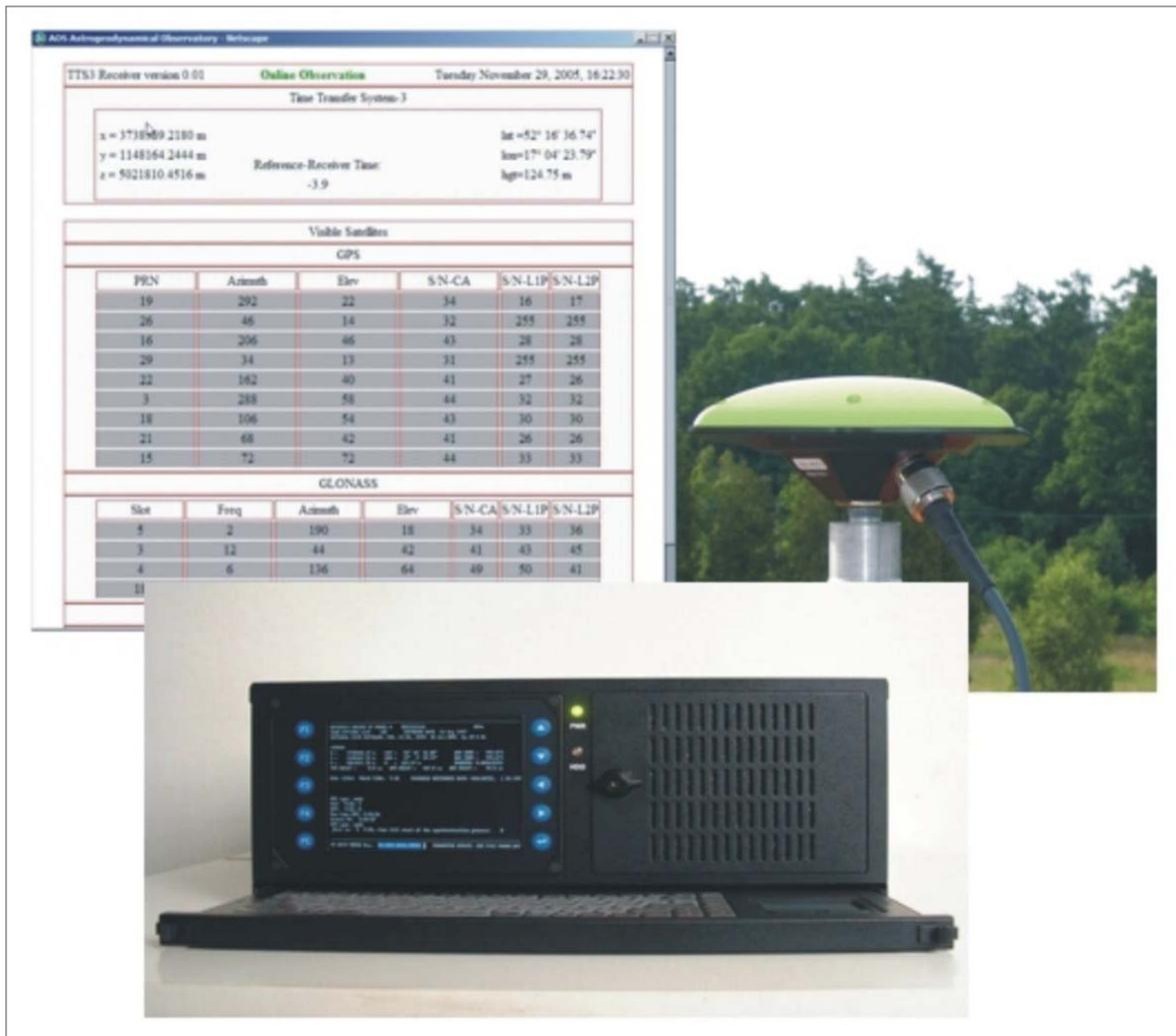
Fig. 4.4.4. TTS-3, Time transfer system developed by the Borowiec Astrogeodynamic Observatory of the Space Research Centre (AOS)
