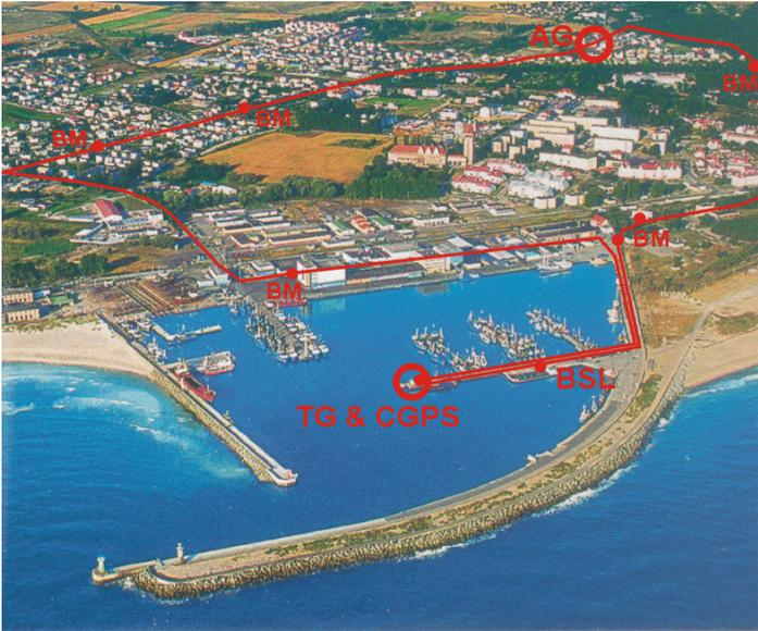
Fig. 1.6.7. Collocation of different observing techniques at CGPS WLAD station
