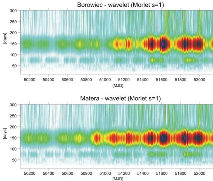
Fig. 4.7.8. Wavelet time-frequency spectrum of the TEC data from Borowiec (a) and Matera (b) during the period of 1996 to 2001 (Krankowski et al., 2005b)
