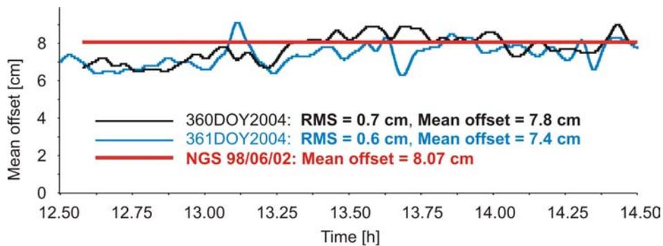
Fig. 4.5.10. The example of mean offset determination
