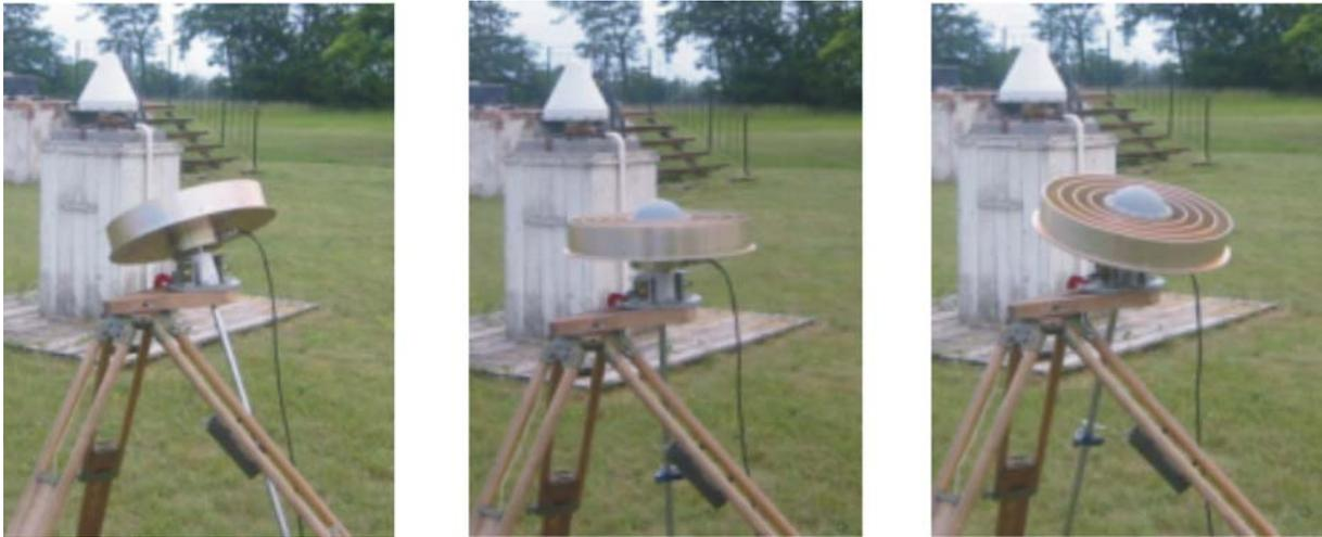
Fig. 4.5.9. The first prototype of portable dynamic tilting device for field calibration of GNSS antenna, checked in the Borowa Gora Observatory
