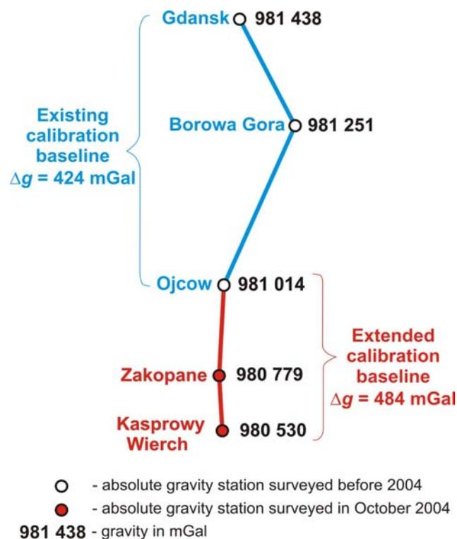
Fig. 2.4.1. Central Gravity Calibration Baseline in Poland (2004)
