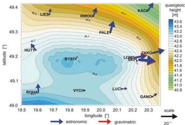
Fig. 2.2.7. Astronomical and gravimetric deflections of the vertical
