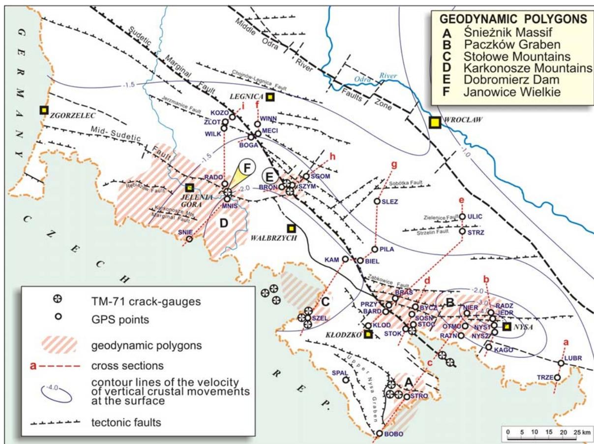
Fig. 3.2.6. Sudety Mountains and Fore Sudetic Block geodynamic areas; GEOSUD network and geodynamic polygons
