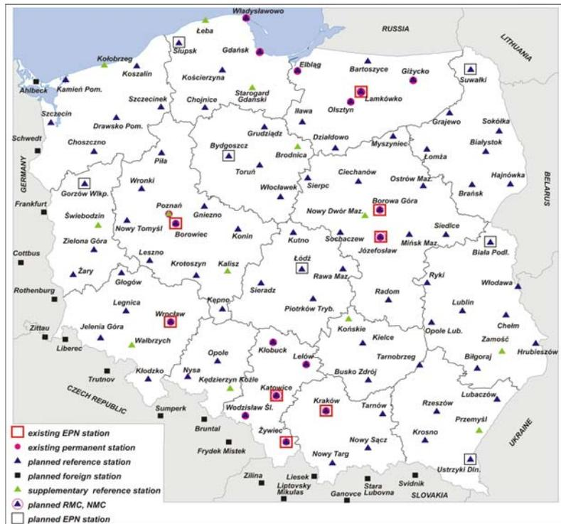
Fig. 1.5.4. Reference stations of the Polish part of the EUPOS network
