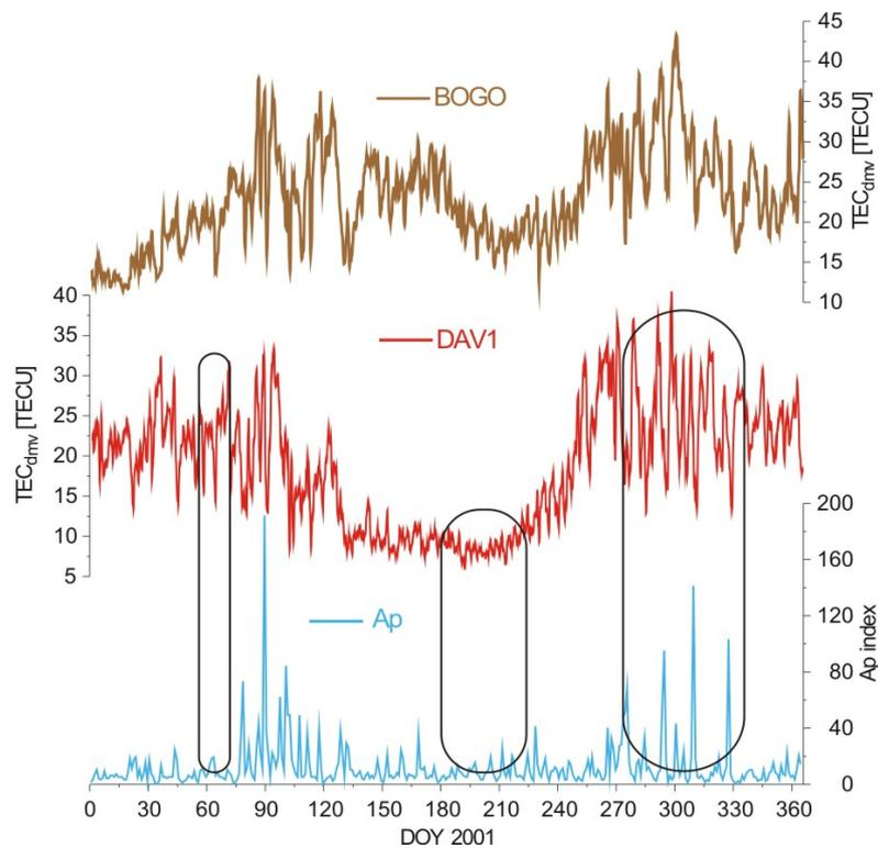
Fig. 4.7.11. The Ap index and annual variations of diurnal mean TEC over DAV1 and BOGO stations obtained from IONEX data
