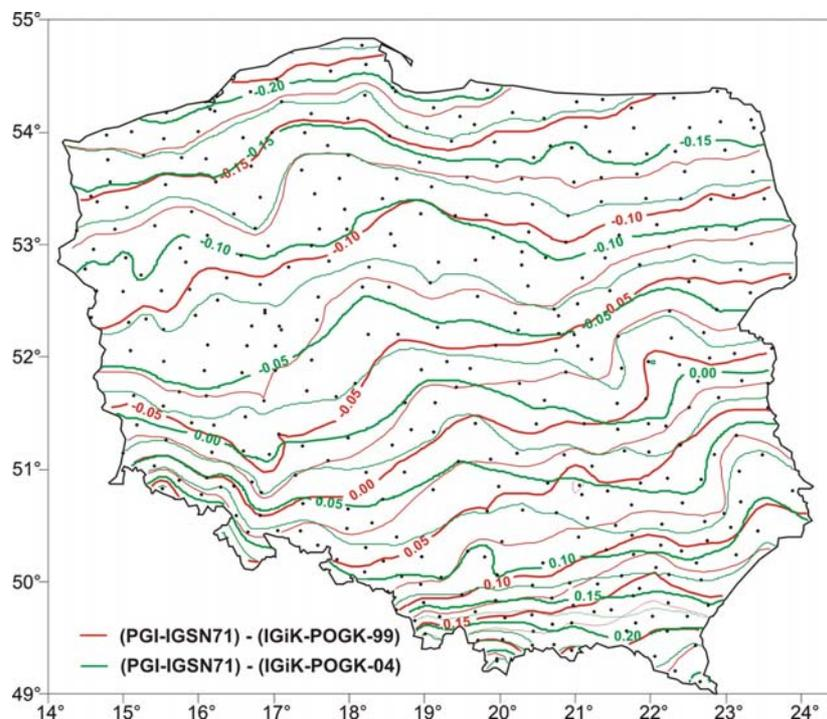
Fig. 1.7.2. Corrections due to transformation from PGI-IGSN71 to IGIK-POGK-99 and IGIK-POGK-04 [mGal]
