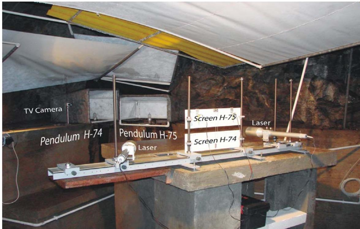
Fig. 3.5.1. New system of registration of quartz horizontal pendulums H-74 and H-75
