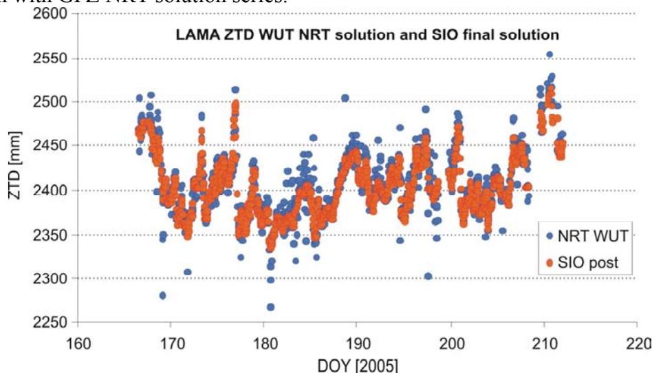
Fig. 4.6.5. Final ZTD solution (global IGS by SIO) and WUT NRT solution
