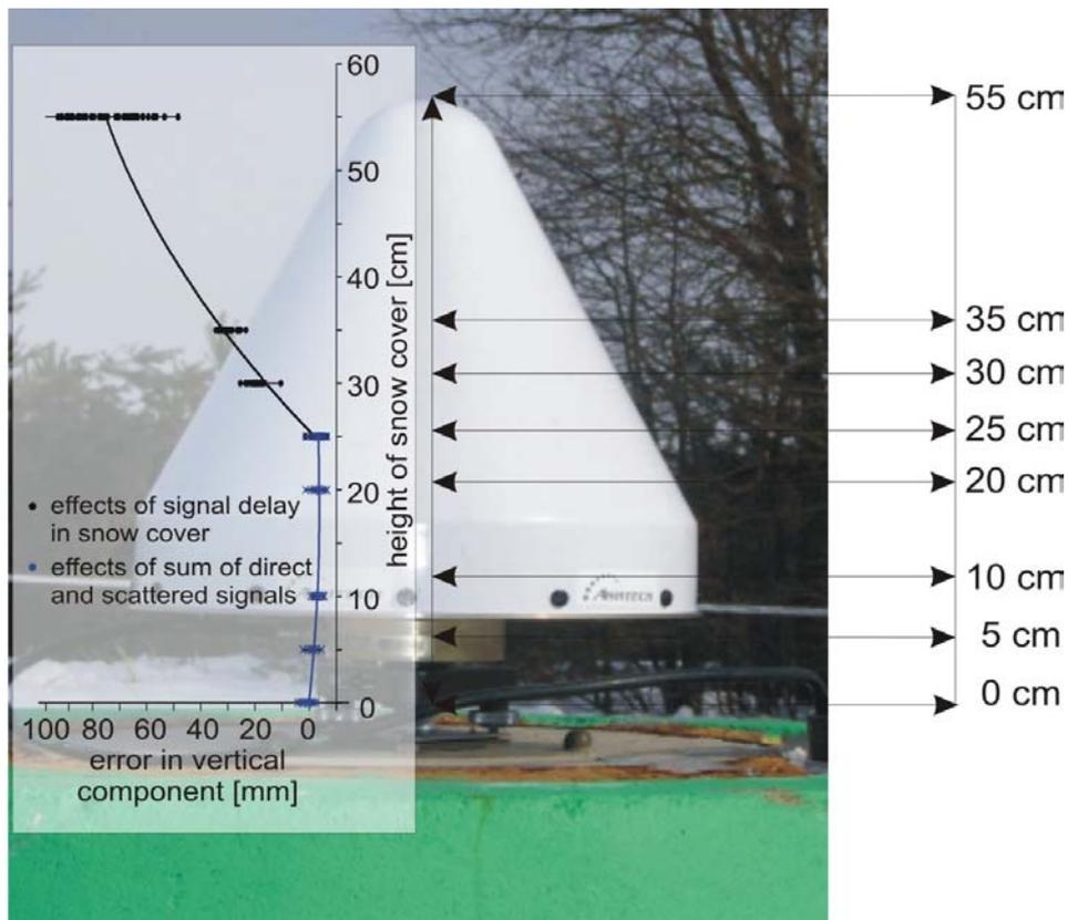
Fig. 4.5.12. Dependence of vertical component determined on the coverage of the antenna with the snow
