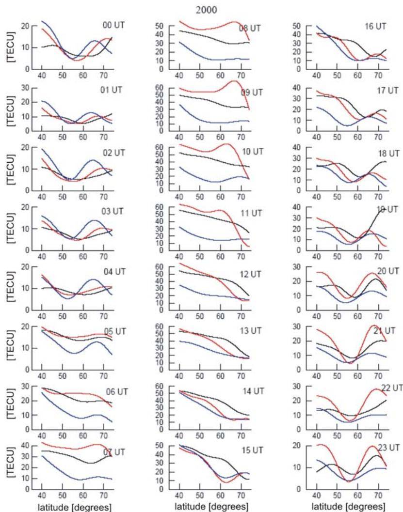
Fig. 4.7.1. Latitudinal TEC profiles over Europe at longitude 20°E. Black line – 2 October ( $\Sigma Kp = 16$ ), red line – 4 October ( $\Sigma Kp = 40$ ), blue line – 5 October ( $\Sigma Kp = 53$ ) (Wielgosz et al., 2004a)
