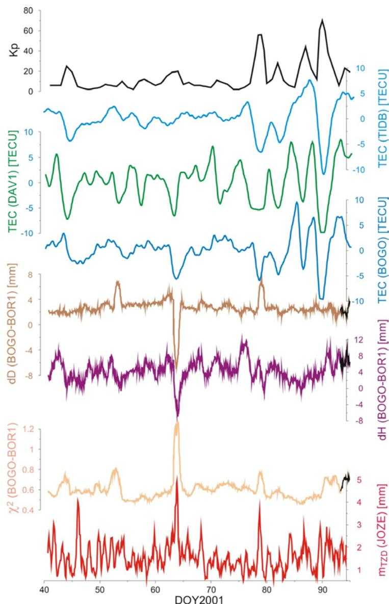
Fig. 4.7.10. Variability of vertical component and the length of BOGO-BOR1 vector as well as  $\chi^2$  against of solar activity Kp, filtered TEC and mean square errors of TZD
