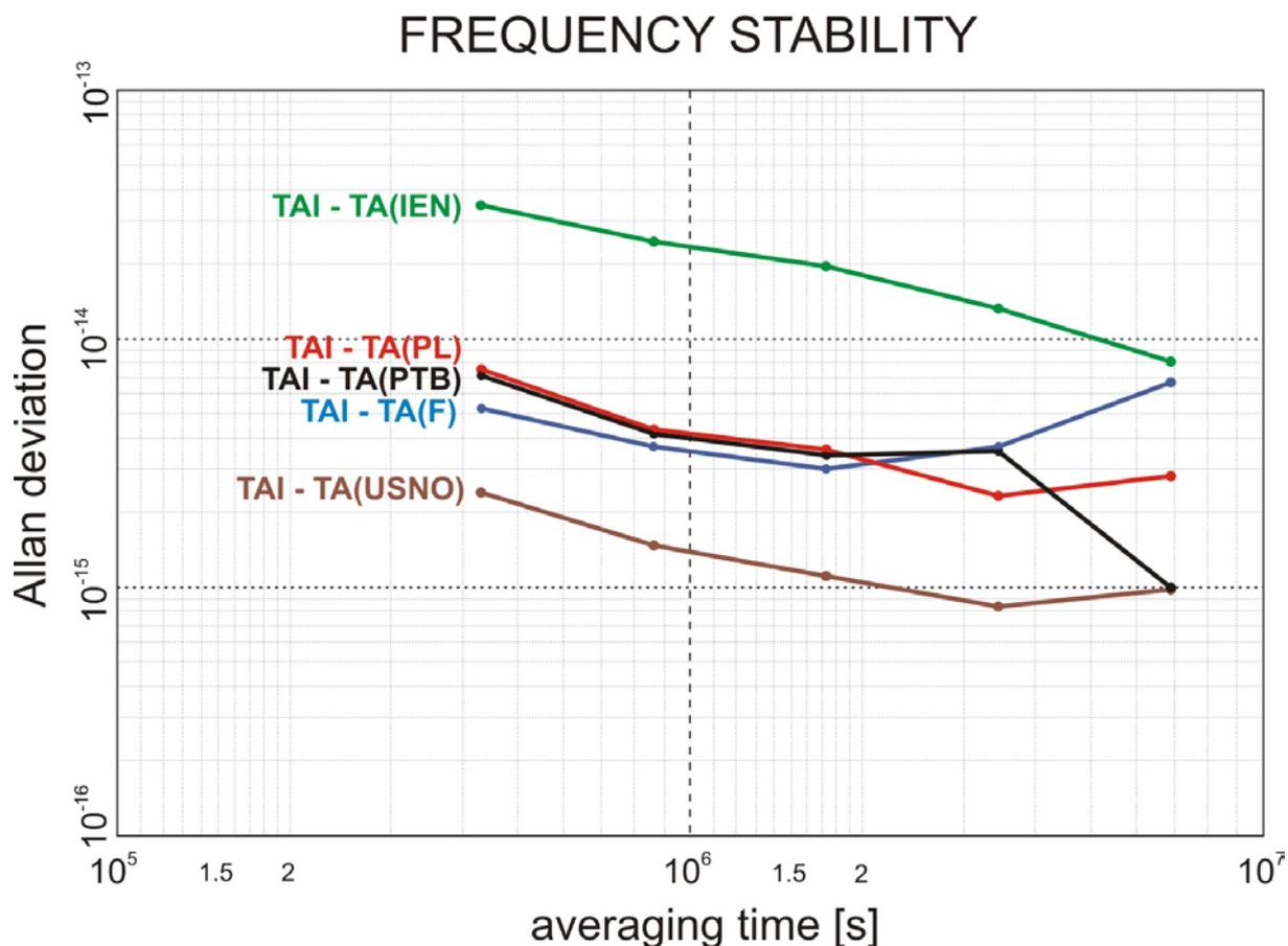
Fig. 4.4.3. Allan deviation analysis of the stability of TA(PL)
