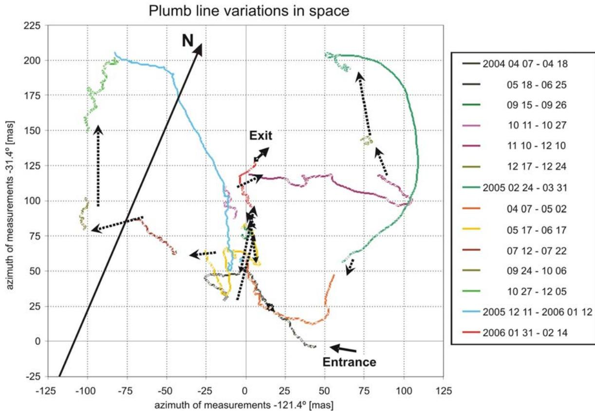
Fig. 3.5.4. Graph of plumb line variations in space during 2004-2005
