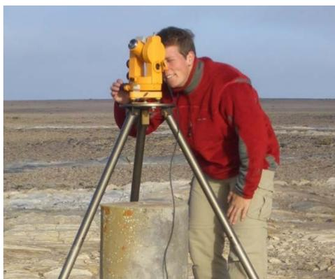
*Measuring the geomagnetic field at a so-called repeat station in Namibia*
